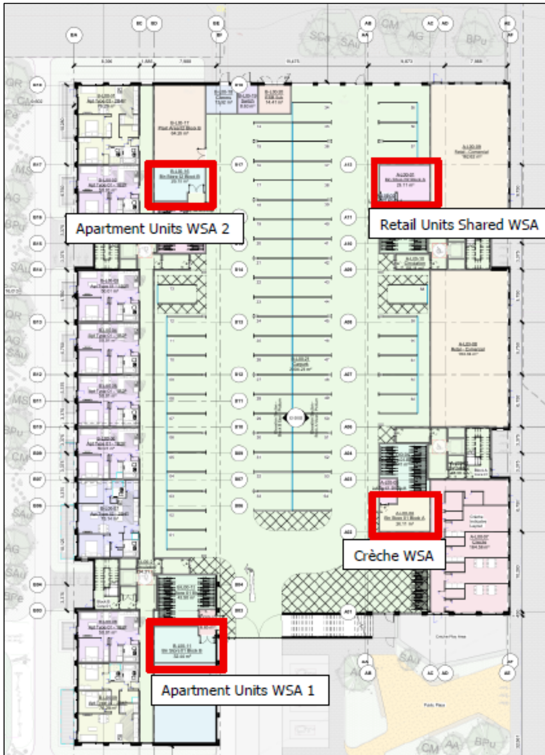
Figure 6-1 Waste Storage Area
