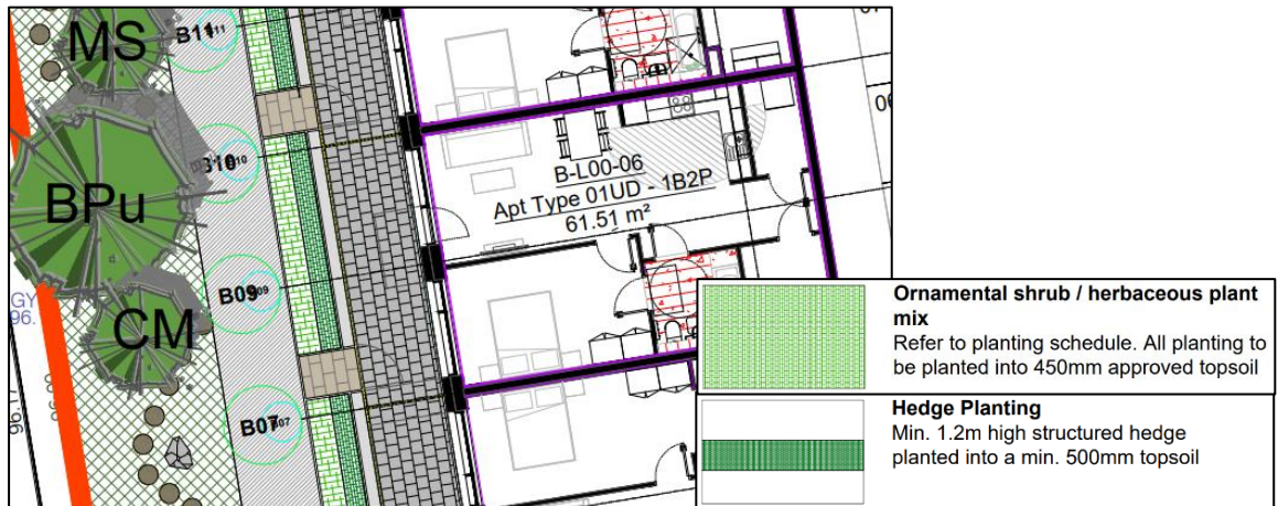
Figure 6.8: Extract from the Landscape Masterplan , showing the ornamental shrub / herbaceous mix planting and a 1.2 m high hedge defining the
