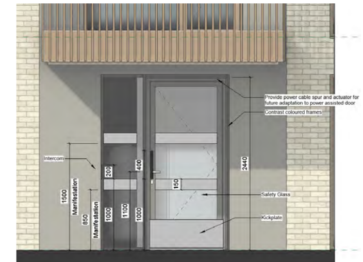
Typical Entrance - Elevation
